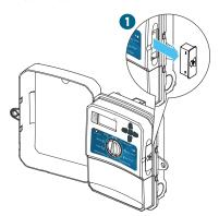
When installed, WAND disables the controller's dial and button functions, the existing schedule, and settings.
